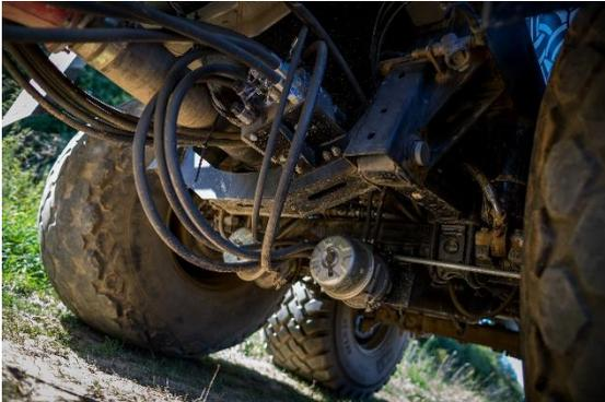
**Picture caption:** With the AGRO Drive hydraulic drive axle from BPW, drawbar trailers are now digging their own way out of the sludge. (Source: BPW Bergische Achsen KG)
