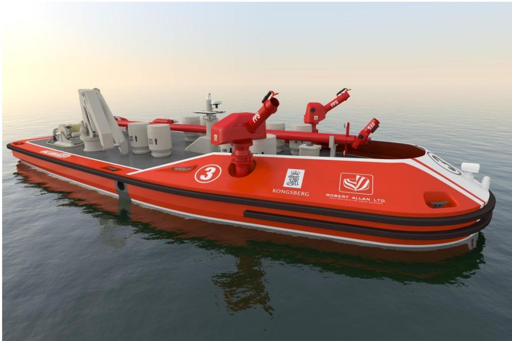
The first in the series will be the 20 m RALamander 2000, equipped with Fi Fi 1 capability, with a total pumping capacity of 2400 m<sup>3</sup>/hr with optional foam
