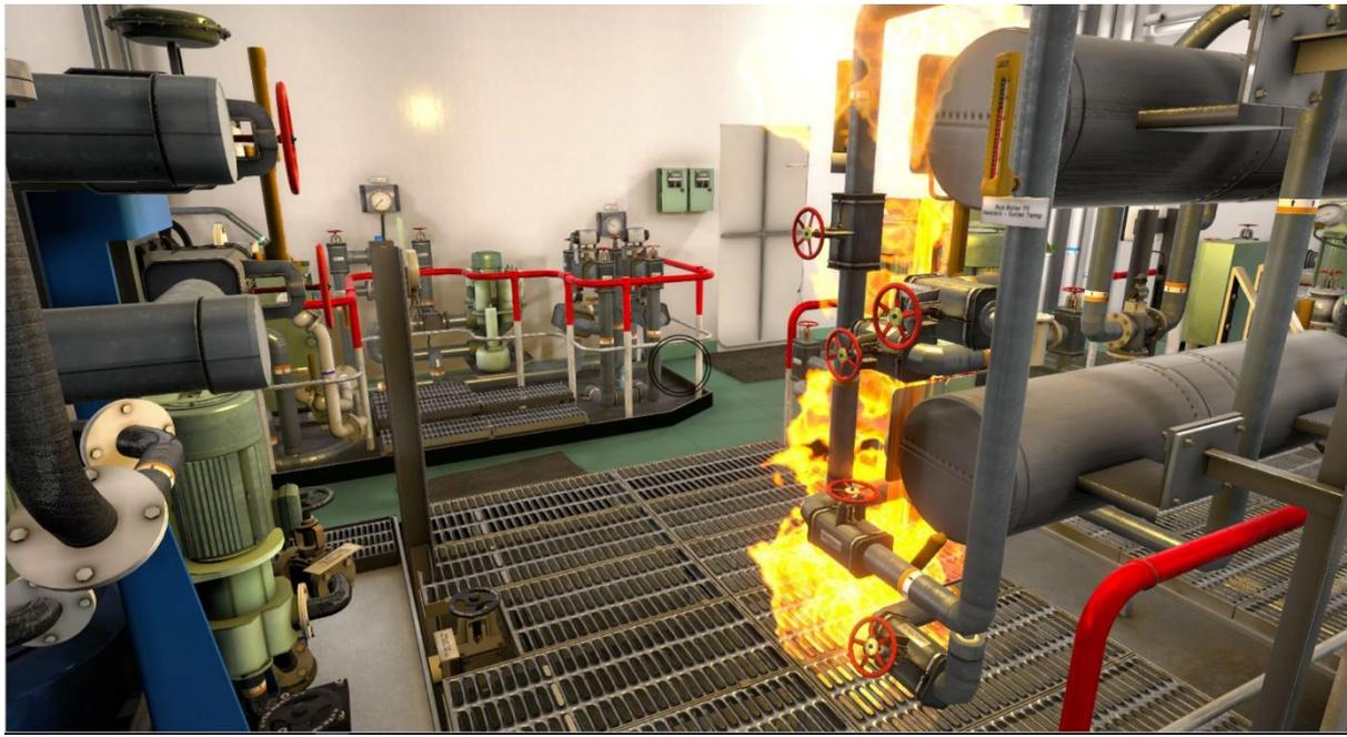
New K-Sim Safety provides an efficient training solution for officers in advanced firefighting. The system includes an interactive 3D walk-through animation of the entire engine room and four upper decks.
