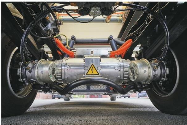
**Picture caption:** Converting existing vehicles to accommodate BPW’s electric drive axle, eTransport, paves the way for zero-emission logistics. (Source: BPW Bergische Achsen KG)
