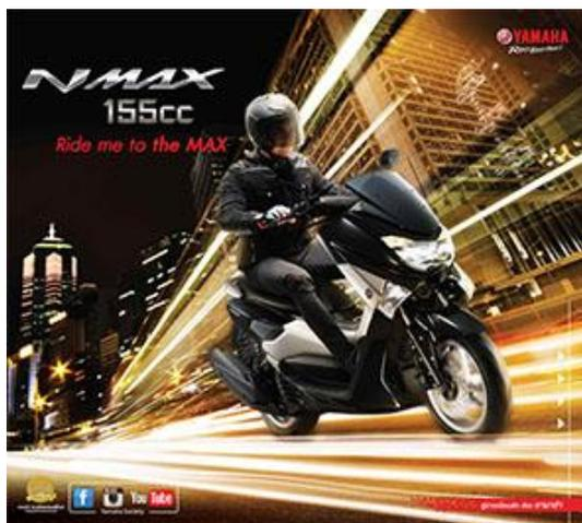
The 2015 NMAX model for markets worldwide is offered in 125cc and 155cc variations with the latest engines that feature a variable valve system that further improves combustion efficiency.
