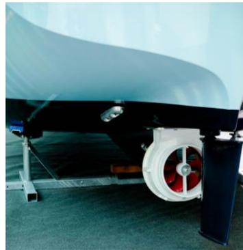
*The VETUS E-POD electric drive solution is mounted in the stern*
