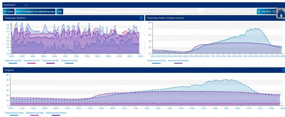
Figure 3 - The temperatures in the refrigerated warehouse are displayed via an informative dashboard - (Image source: Kühlmann)
