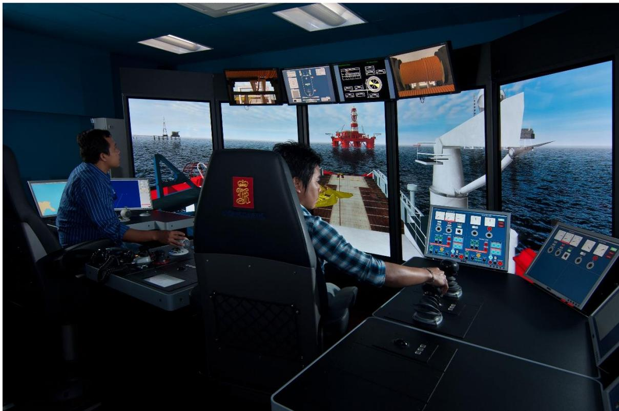
K-Sim Offshore with integrated Kongsberg Dynamic Positioning system is specially designed for advanced offshore operations and will be vital in JMI's future training programs.
