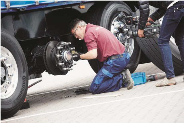
Caption: The ECO Disc brake produced by BPW allows pads to be changed in record time. (Source: BPW Bergische Achsen KG)
