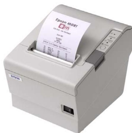
Epson TM-T88IV thermal receipt printer
