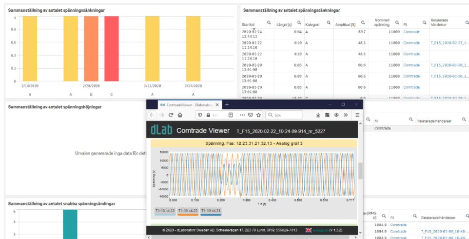
Figure 5: Voltage variations dashboard viewing the waveform of a voltage dip
