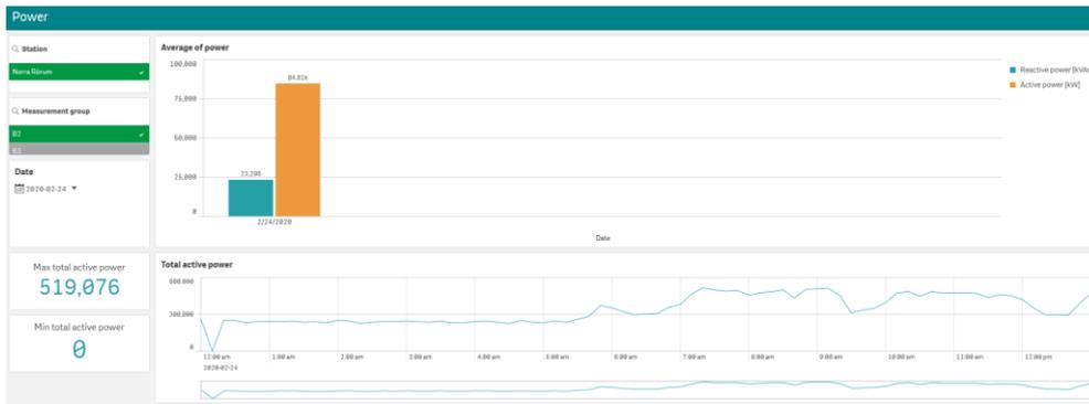
Figure 1: Power graphs for a feeder of a substation. An average over the chosen time is shown in the bar graph, and the 10-minute values are shown in the line graph.
